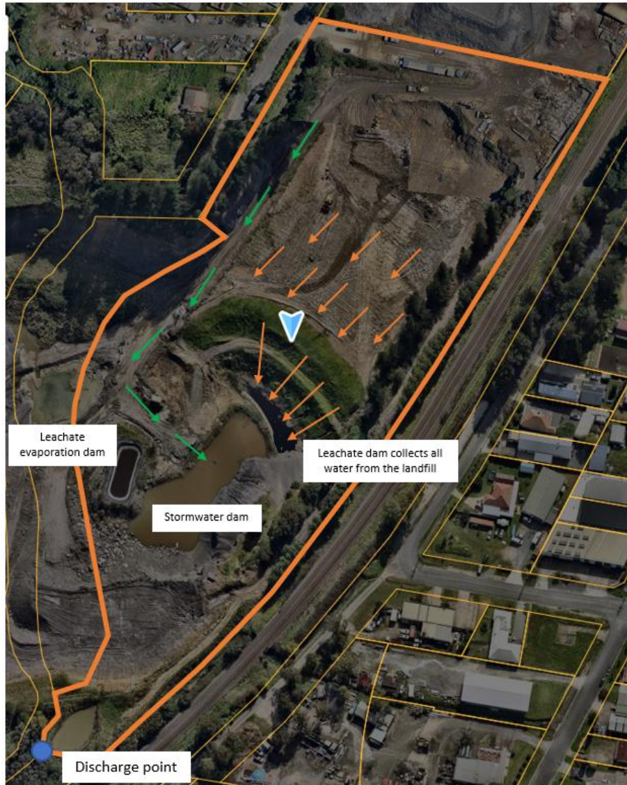
Figure 2: Site Stormwater Directional Flows
