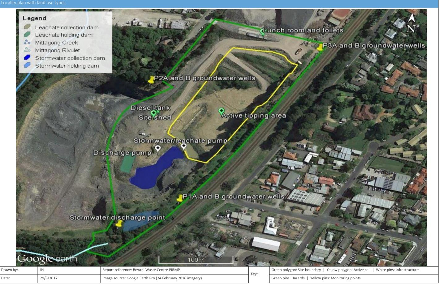
Figure 2: Site plan, showing the location of key hazards identified in this Plan.
